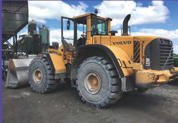
Location: a limestone quarry in Ireland Equipment: Volvo L220F Tire: WESTLAKE CB790
