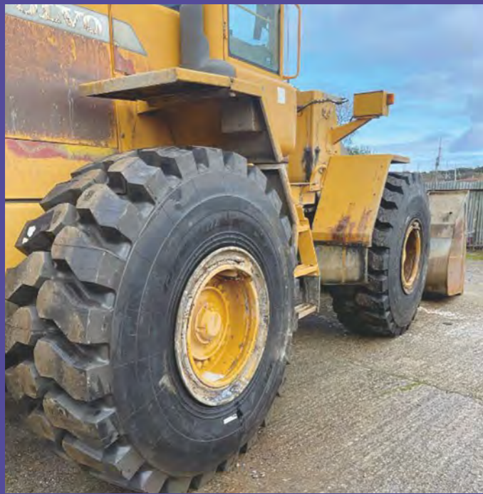
Location: a quarry in UK Equipment: Volvo L120 wheeled loader Tire: WESTLAKE CB773
